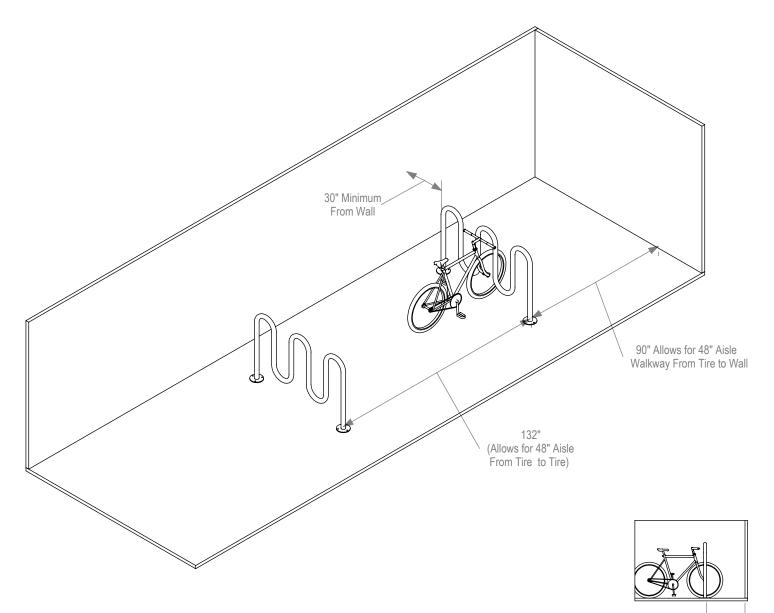
30" Allows for Tire Clearance to Wall
