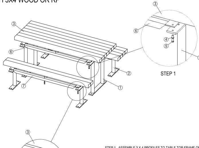
STEP 1 ASSEMBLE 3 X 4 PROFILES TO TABLE TOP FRAME OR TABLE TIE AND TABLE LEGS WITH WASHERS AND LAG BOLTS.
