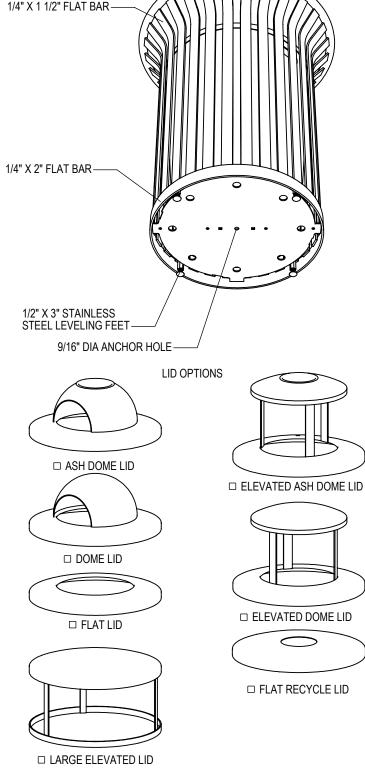
TRASH LIDS ARE ATTACHED WITH STEEL VINYL COATED AIRCRAFT CABLE. PLASTIC LINER INCLUDED. ALL FASTENERS ARE STAINLESS STEEL.
