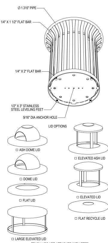
TRASH LIDS ARE ATTACHED WITH STEEL VINYL COATED AIRCRAFT CABLE. PLASTIC LINER INCLUDED. ALL FASTENERS ARE STAINLESS STEEL
