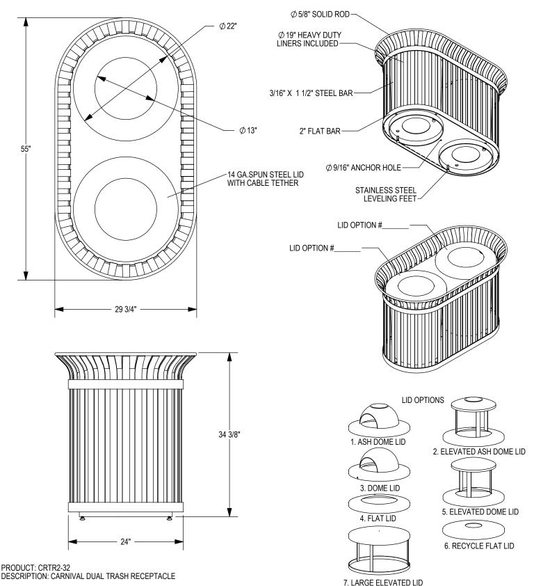
SITE FURNISHING IS POWDER COATED WITH TGIC POLYESTER. STEEL SURFACE PREP INCLUDES MECHANICAL AND CHEMICAL ETCHING FOLLOWED WITH A COATING TO IMPROVE ADHESION AND CORROSION RESISTANCE.
