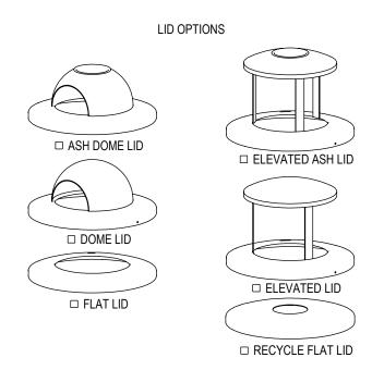
TRASH LIDS ARE ATTACHED WITH 2 EA. STEEL VINYL COATED AIRCRAFT CABLE. PLASTIC LINER INCLUDED. ALL FASTENERS ARE STAINLESS STEEL
