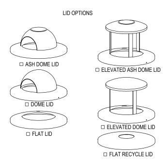
TRASH LIDS ARE ATTACHED WITH 2 EA. STEEL VINYL COATED AIRCRAFT CABLE.
