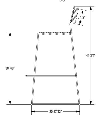
SITE FURNISHING IS POWDER COATED WITH TGIC POLYESTER. STEEL SURFACE PREP INCLUDES MECHANICAL AND CHEMICAL ETCHING FOLLOWED WITH A COATING TO IMPROVE ADHESION AND CORROSION RESISTANCE.
