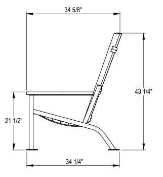
STEEL FRAME CAN BE FINISHED WITH POWDER COAT PAINT OR HOT DIP GALVANIZE.
