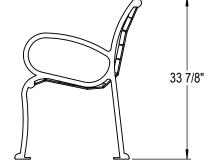
SITE FURNISHING IS POWDER COATED WITH TGIC POLYESTER. STEEL SURFACE PREP INCLUDES MECHANICAL AND CHEMICAL ETCHING FOLLOWED WITH A COATING TO IMPROVE ADHESION AND CORROSION RESISTANCE.
