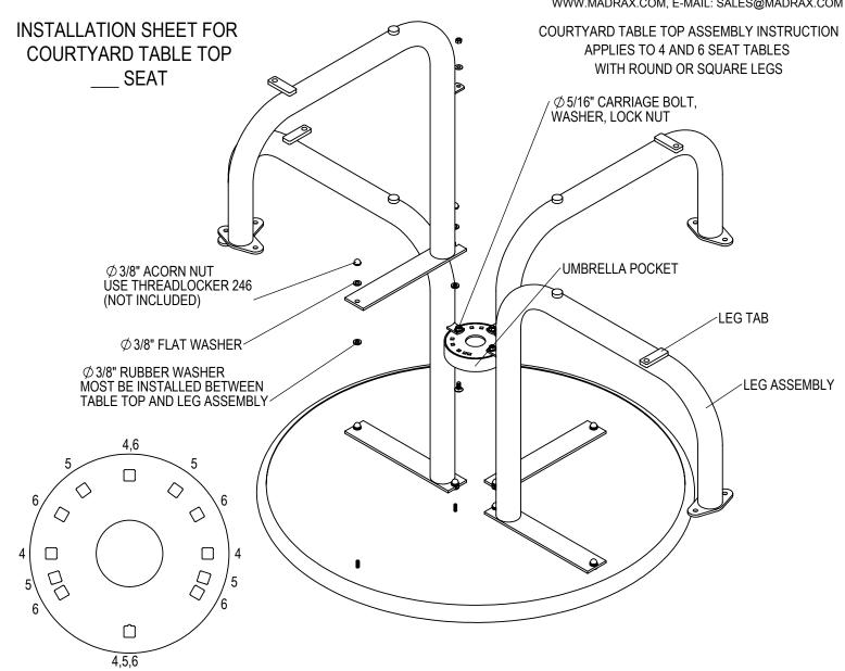
ALL FASTENERS MUST BE HAND TIGHTENED. DO NOT OVER TORQUE. LEAVE LOOSE UNTIL FULLY ASSEMBLED.
